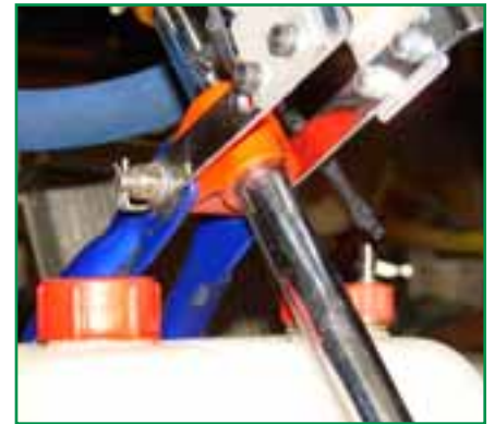
Put a mark on the steering shaft and upper steering support to identify straight ahead. This will be important when scaling your kart.
