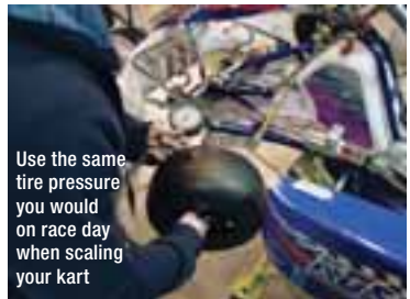
The circumference of the front and rear tires should be within 1/4" in of each other.
